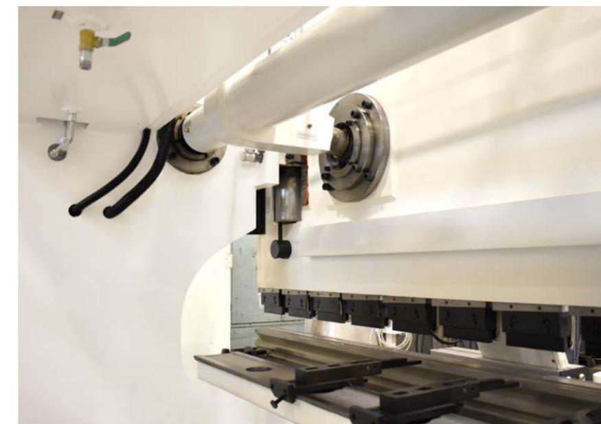
Torque tube/X-axis back gauge
