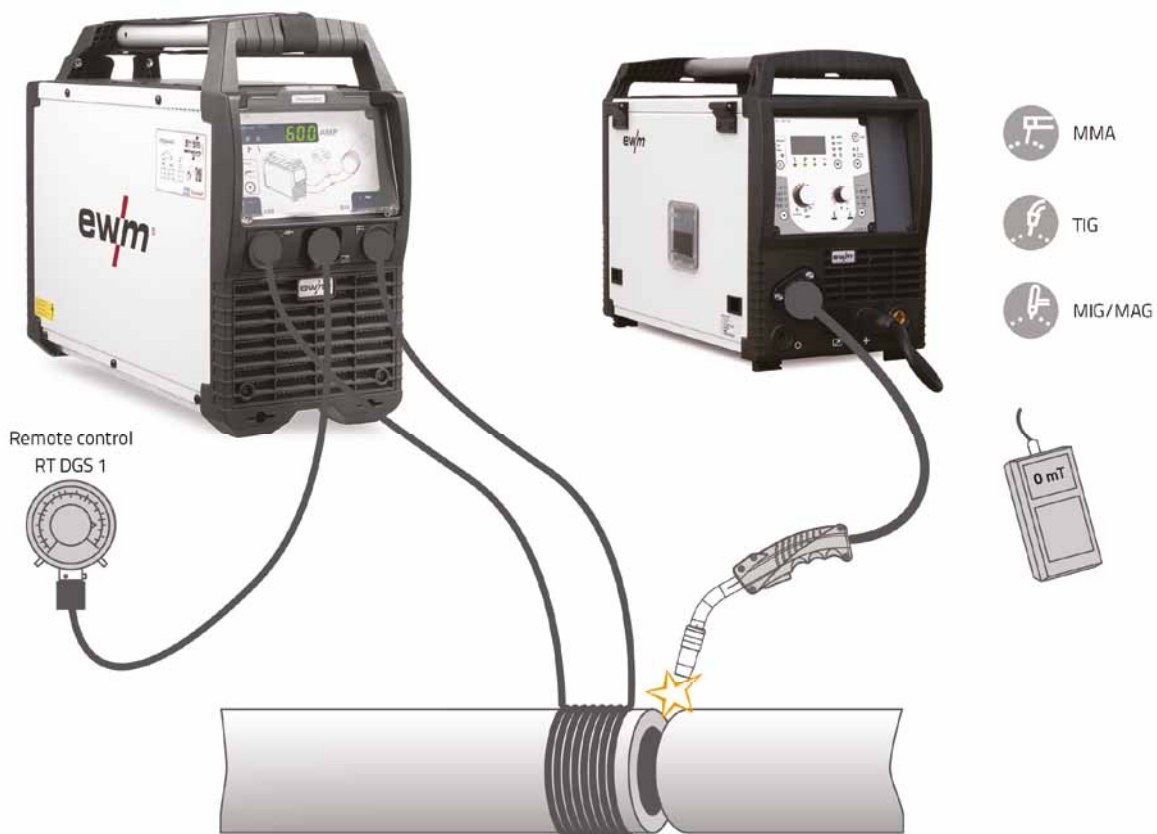
Degaussing during the welding process
