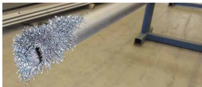
Fig. 6 Filings arranged in a Christmas tree pattern are an indication of magnetism
