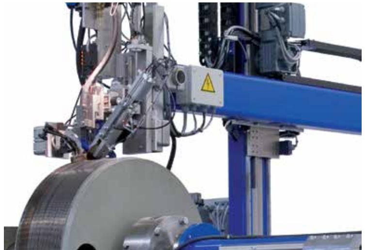
Automated welding head
