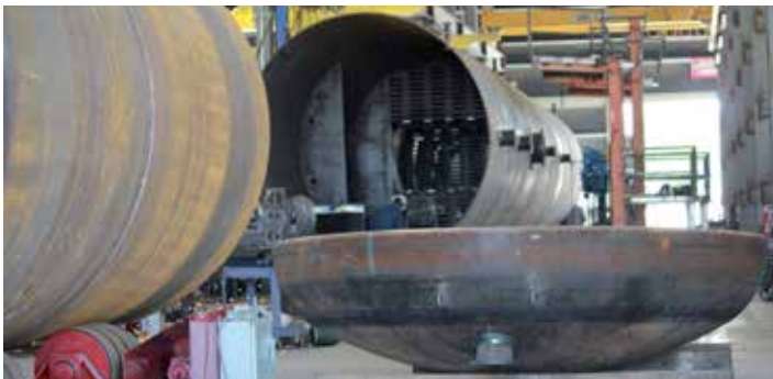
Pressure vessel construction
