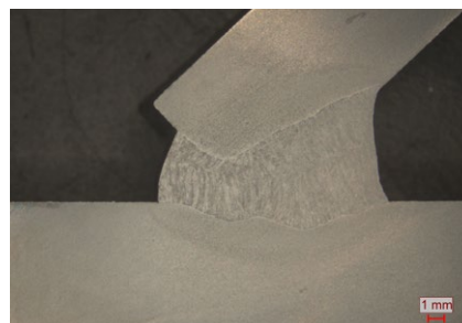
Web plate material thickness 10 mm, included angle 35°
