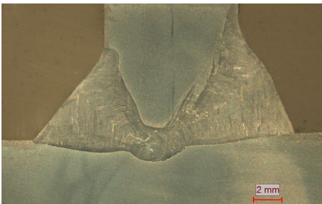
PB Full penetration, welded on both sides
