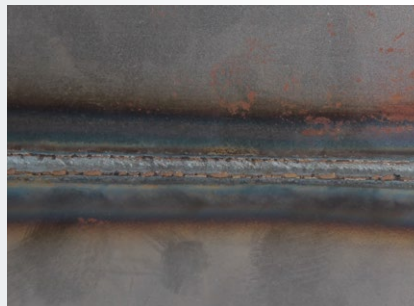
S355, material thickness 3 mm, using G3Si1 1.2 mm diameter at 100% CO 2
