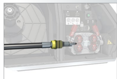
Connection for drum feed
