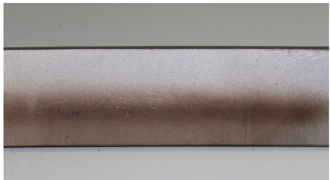
Back view: Low heat input using forceArc puls ® , less surface oxidation
