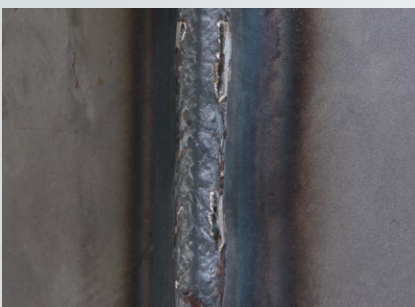
S355, material thickness 3 mm, using G3Si1 1.2 mm diameter at 100% CO 2
