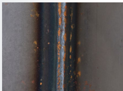
S355, material thickness 3 mm, using G3Si1 1.2 mm diameter at 100% CO 2
