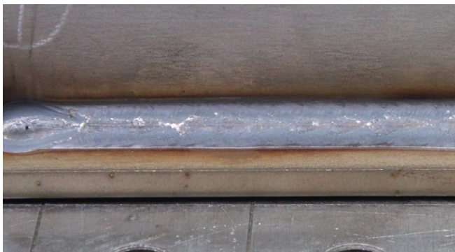
Front view: Lower heat input using forceArc puls ® , less surface oxidation resulting in a better finish
