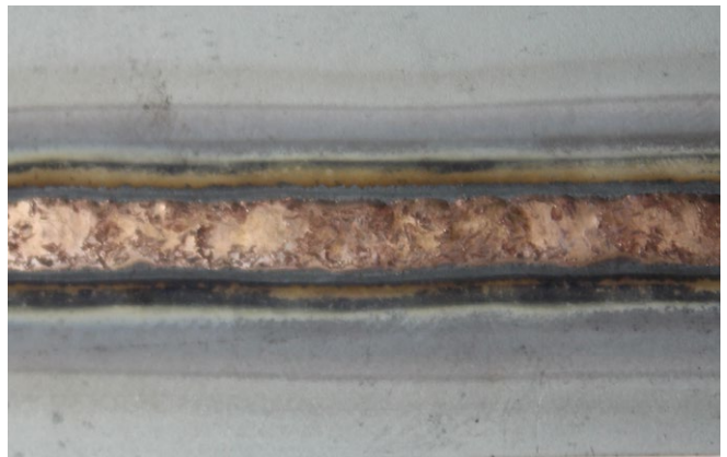
Brazing galvanised sheet metal
