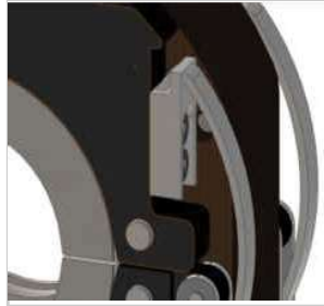
Adjustable spring loaded system: accounts for tube "out of round"
